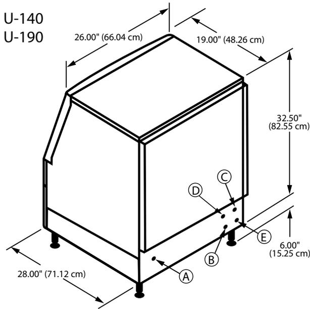
**Installation Note** Recommended clearance for top, sides, and back is 5" (12.7 cm) however, there is no minimum clearance required.
