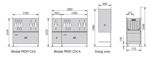
Loading height: 440 mm Loading width: 510 mm
