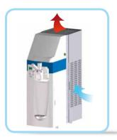
Vertical venting to reduce the machine's footprint
